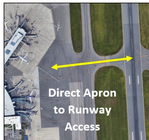
Figure 4-10 – Direct Apron-to-Runway Access
